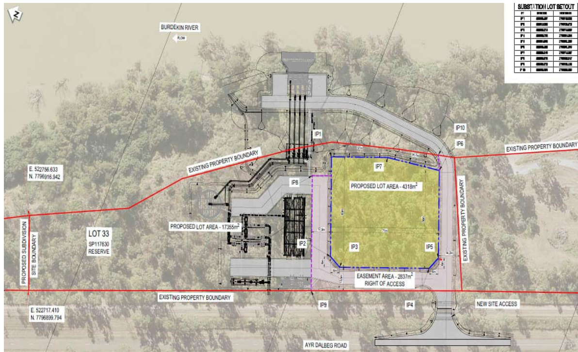
Figure 4 Substation Site Layout
