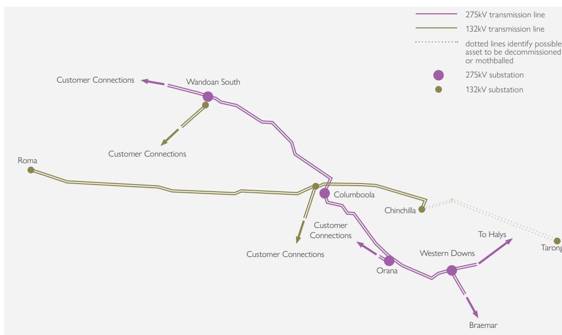
Figure 6.15 Surat Basin North West area transmission network
