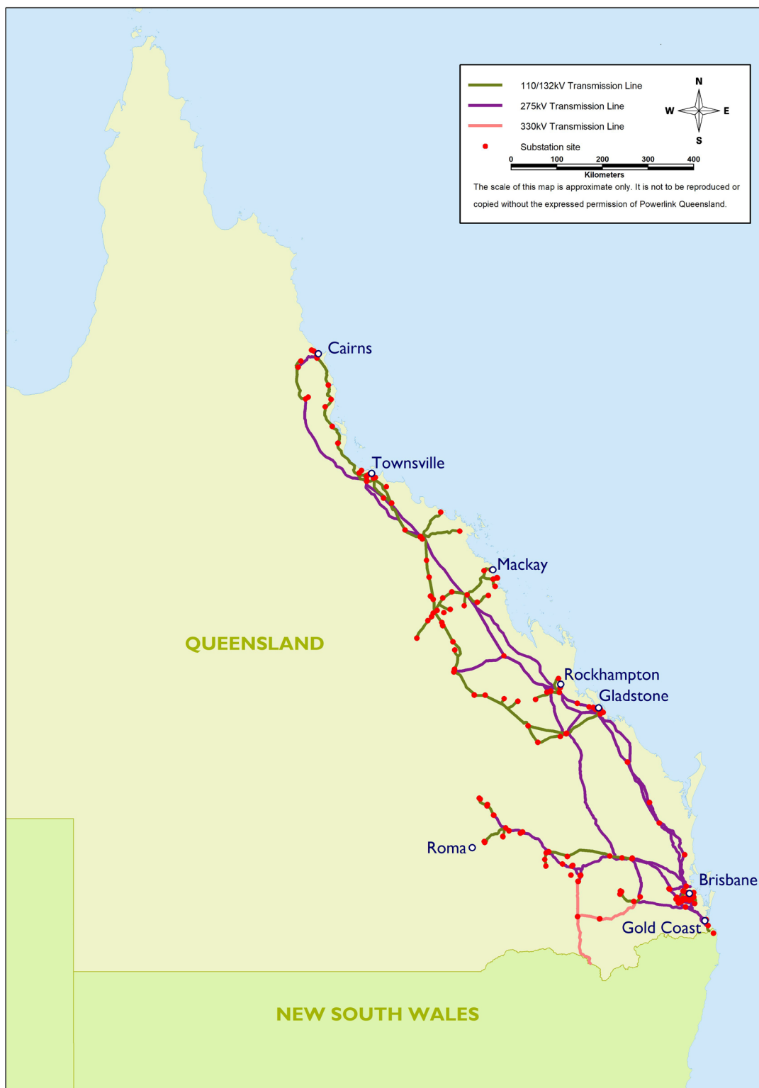
Figure 9.1 Existing Powerlink Queensland transmission network October 2024
