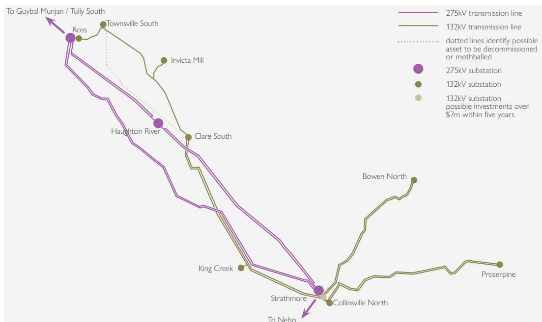
Figure 6.10 Southern Ross zone transmission network
