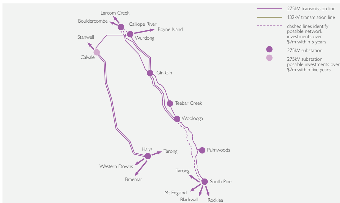
Figure 6.14 CQ-SQ transmission network
