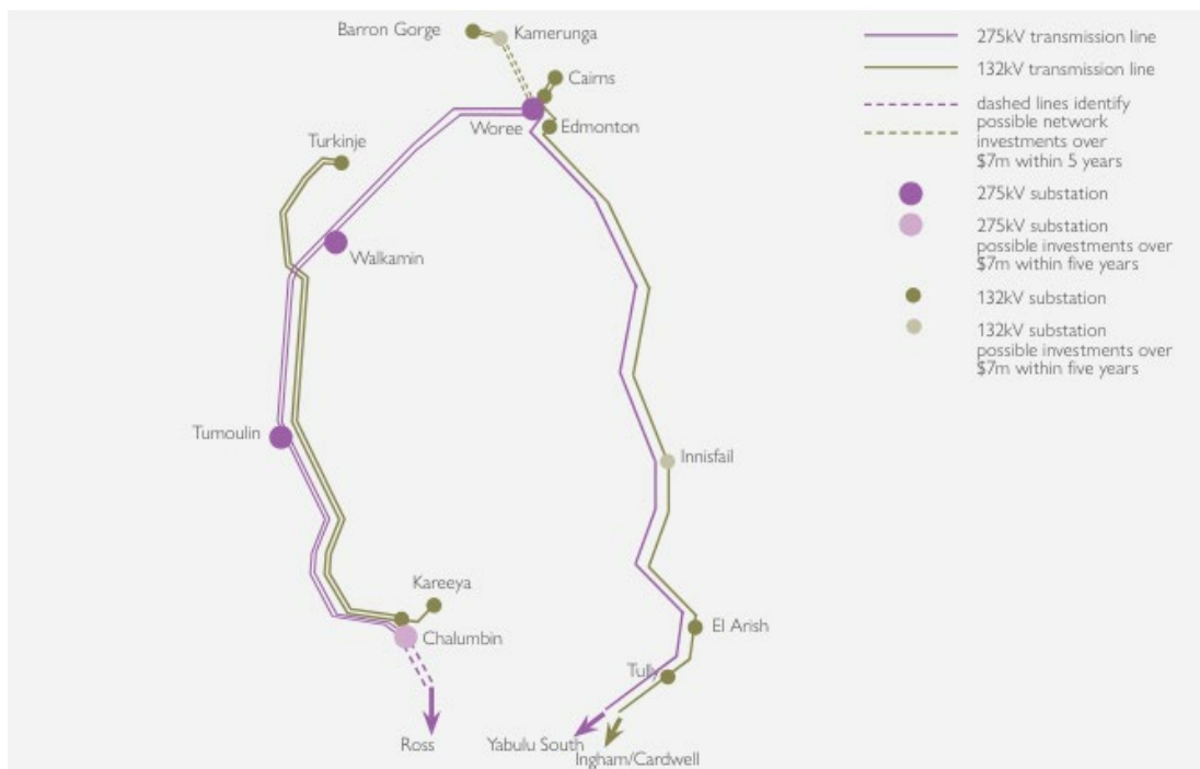
Figure 3.1: Far North zone transmission network
